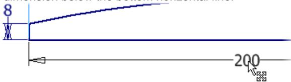
9) The sketch dimensions are parametric, meaning that the value of the dimension controls the size of the geometry. Change the size of the 200 mm by double-clicking on it and enter **250** in the Edit Dimension dialog box and then press Enter or click the green check mark in the dialog box.
